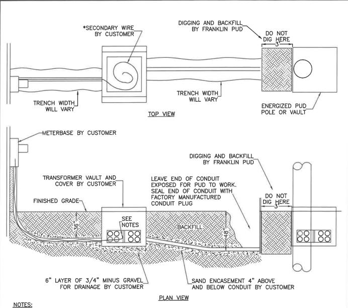
\* LOOP ENOUGH SECONDARY WIRE SLACK IN VAULT TO ALLOW CABLE TO EXTEND 8' ABOVE VAULT COVER. CHECK WITH FRANKLIN PUD ENGINEERING FOR SECONDARY DETAILS.
