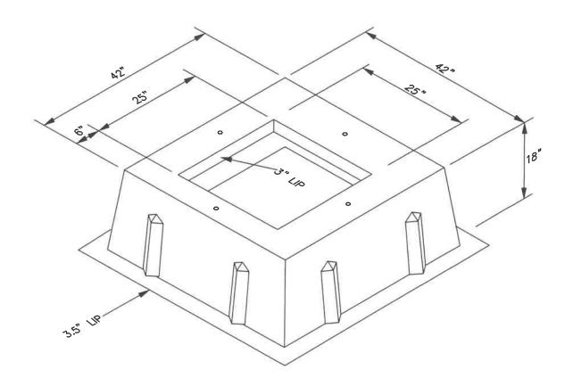
1) VAULT, FIBERGLASS - 42"x 42"x 18" DEEP WITH 25"X 25" OPENING.
